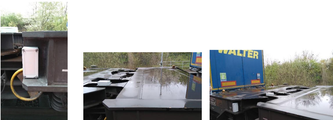
Figure 13: Mounted GPS tracker on different train wagons
